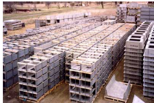
Fig 15 Pipe Trench Liners, USA
