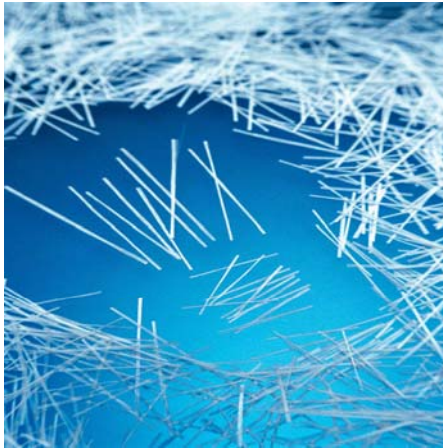
Fig 1A AR Glass Fiber Chopped Strands
