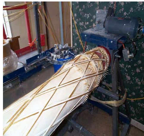
Fig 3 Filament Winding of a pole with AR Glass Fibers
